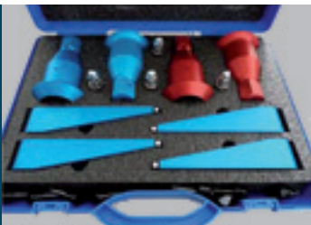
Central locking VAS 6828* Central locking with spoiler adapter, for the Porsche Carrera GT.
