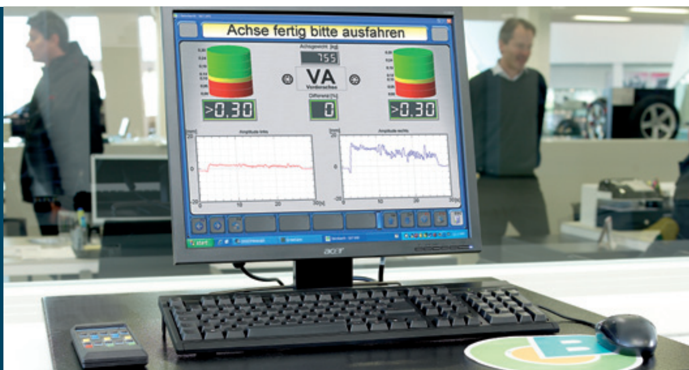
Accurate, clear display of the determined values with amplitude for both absorbers.
