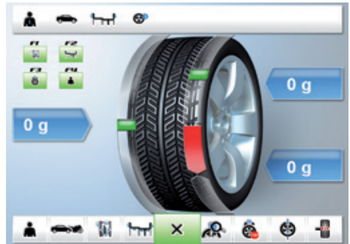
Facilitates the work: Indication of the weight placement (hidden gluing) behind the spokes.
