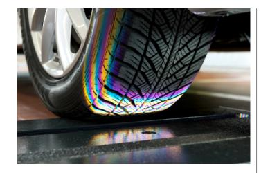
High torque and heavy batteries lead to extreme tire wear, especially in electric vehicles. In addition to tread depth, we also assess uneven wear patterns as the vehicle drives over the system, allowing us to detect potential chassis and tire pressure issues within seconds.
