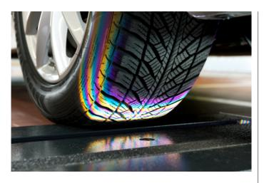
High torque and heavy batteries lead to extreme tire wear, especially in electric vehicles. In addition to tread depth, we also assess uneven wear patterns as the vehicle drives over the system, allowing us to detect potential chassis and tire pressure issues within seconds.
